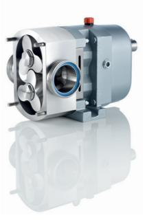
With its unique three-wing rotor design, the FL3 greatly expands the application range of Fristam's FL positive displacement pumps. Its helical rotors virtually eliminate pulsation, ensuring gentle product handling while allowing higher transfer capacity and superb CIP.
